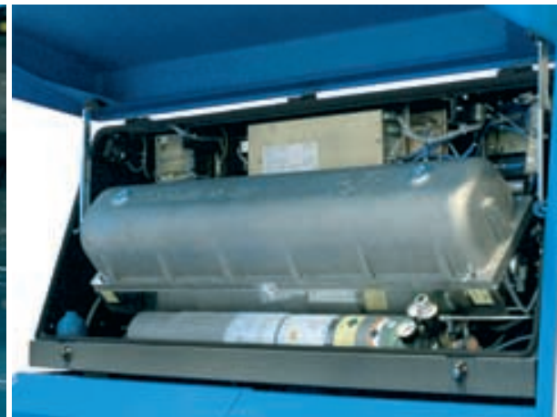
Diffusion cooled CO 2 SLAB Laser
